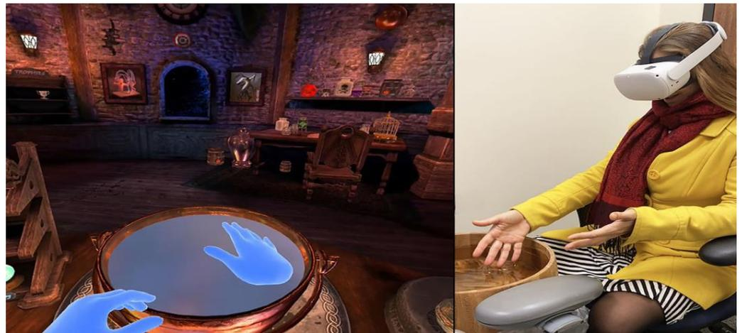
**Figure 4.** Above right is a photo of the Meta Quest2 VR helmet. This lightweight helmet weighs only 17.7 ounces, is wireless, and uses cameras to optically track head and hand movements. Image on left shows a screenshot from an optically hand-tracked game named *Waltz of the Wizard*, aldin.com, accessed on 28 November 2022, photo on right by Hunter Hoffman, both images copyright Hunter Hoffman, [www.vrpain.com](http://www.vrpain.com), accessed on 28 November 2022.
